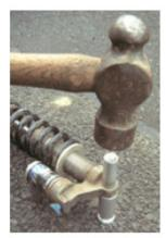
Tap the end of the Bush Drift firmly to knock the new DU Bush into the eyelet of the shock
