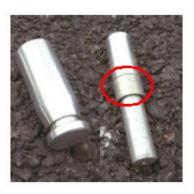
Slide the new DU Bush onto the Bush Drift and the Foot into the tapered end of the Support Sleeve. The foot is there to prevent you damaging the thin end of the Support Sleeve.
